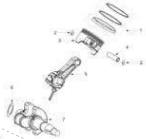
FIG.5 : RING SET,OIL / ROD,CRANKSHAFT CONNETING
